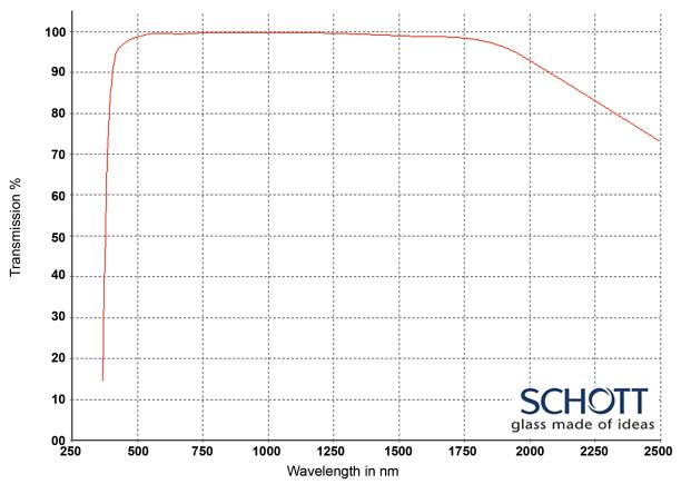
Internal transmittance for 10mm thickness
