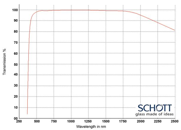
Internal transmittance for 10mm thickness
