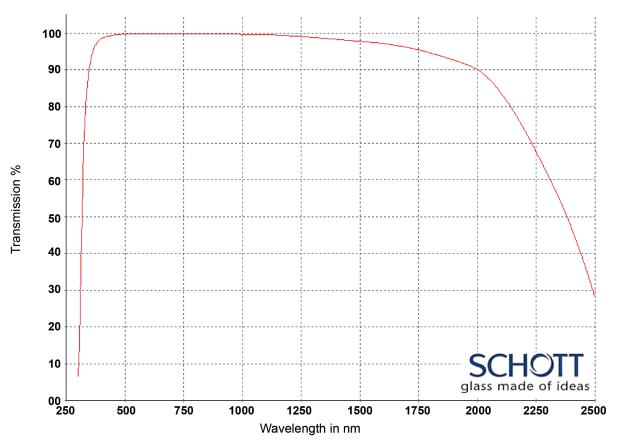
Internal transmittance for 10mm thickness
